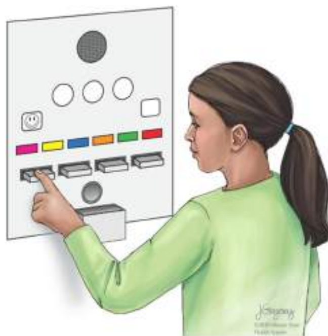
Fig. 1. Diagram of child positioning and the operant test panel. Illustration by Jill Gregory used with permission of ©Mount Sinai Health System. Starting at the top of the panel, there is a speaker and below that, there are three circular press-plates. Below the circular press-plates, there are two different types of stimulus lights - correct and incorrect response indicator lights (smiley face) and serial position indicator lights (colored rectangles). At the bottom of the apparatus, there was a container where a dispenser mounted inside the wooden cabinet delivered nickels.
